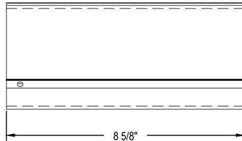
Sleeves are constructed of extruded aluminum tubing with an approximate inside diameter of 3 1/2" and outside diameter of 4". Suitable for installing a 3 1/2" diameter volleyball post in a 4" diameter socket. The sleeve length is approximate 8 1/2". Three 1/4" diameter threaded holes allow setscrews (provided) to attach the sleeve to either the 3 1/2" pole or to the inside diameter of the 4" floor socket or can be used without attachment.
